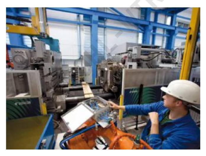
a die casting installation for E-mobility parts with already set-up die casting mould. Set-up times can be decreased relatively easy by approx. 60 %, according to Mr Dr. Krapohl.
